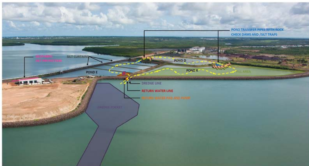
Figure 3. Pond System and Decant Water Flow as originally envisaged in the DDSPMP (approved 2 October 2012)
